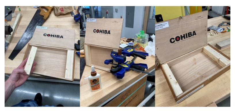
With the neck fully fretted and configured with tuners, the remaining steps were to set the nut into the neck, secure the neck to the cigar box, and then finally configure the bridge/strings. Before the neck could be secured to the box, the box needed to be seriously reinforced. The box in its original form had no solid place to drill any wood screws into, so pieces of scrap wood were cut to size and glued into the box to provide structural integrity.
